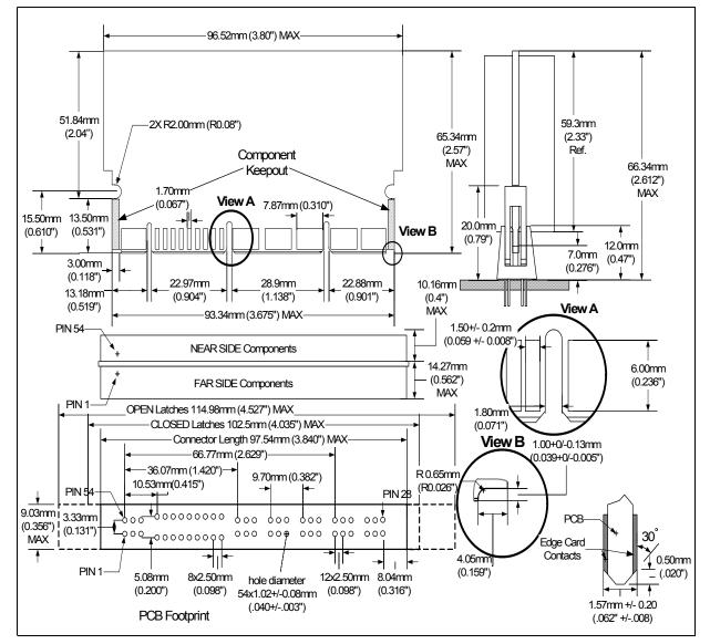
Figure 7-1. VRM 11.0 Module and Connector
